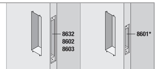
\*If using a 8601 passage mortise, the trim plates may be positioned anywhere on the door, as the trim does not interact with the mortise box.
