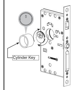
Note: Notches on cylinder must be parallel with the horizontal plane when screwed flush into lock body.
